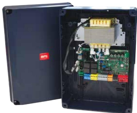
Control panel with dip switches and potentiometers for one or two 24V operators for swing gates
