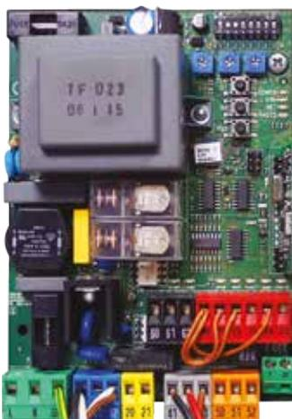
Control panel for DEIMOS AC sliding gate operator range.
